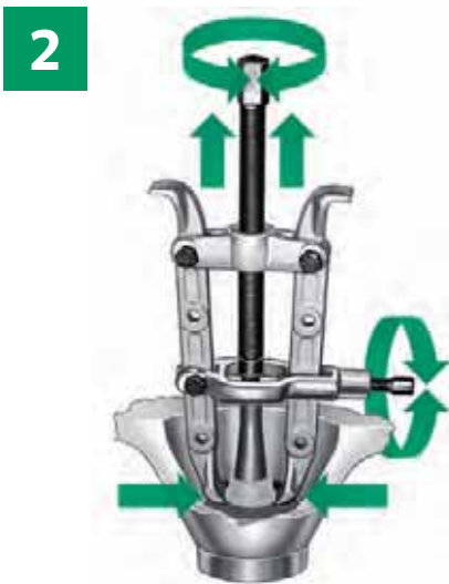
How a two-armed puller works
