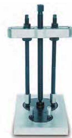
Puller in use for removing gearwheels
