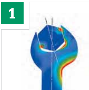
1 Load zones in standard-quality spanners
